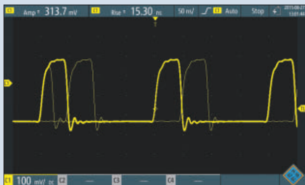
◀ Fig. 3 The high speed acquisition system of the R&S Scope Rider captures up to 50,000 waveforms each second and uncovers rare and unexpected signal anomalies.
